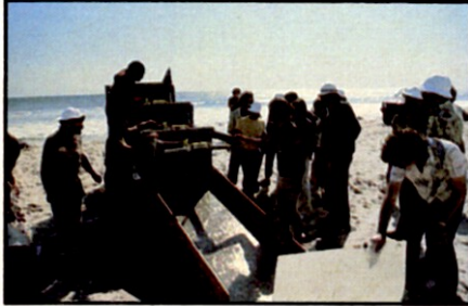
Right: Gaylen Ross faces the onrushing tide while buried in wet sand, the same fate that befalls her lover, Ted Danson (inset top) in "Something To Tide You Over." Although filmed on a real beach, the rushing waters were provided by a homemade "wave machine" (inset above), a sharply inclined metal chute fitted with three large water tanks.
